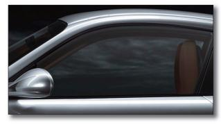
For all of the glass surfaces, including the windshield, Porsche uses a special heat-insulating coating that helps prevent excessively high temperatures inside the vehicle.
