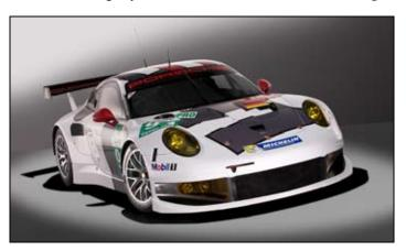
The front and rear mudguards, front and rear lids, doors, underbody, wheel arches, rear wing, dashboard and centre console are constructed from the very light and strong material. Moreover, all windows are made of particularly thin and light polycarbonate.
